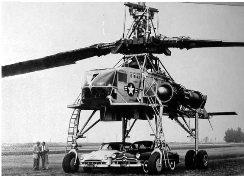
The propulsion system was unusual. Two General Electric J35 turbojet engines were used, sending bleed air up through the rotor hub. The blades were hollow, and the hot compressed air traveled through the blades to tip jets where fuel was injected. In flight the rotors spun at a sedate 88 rpm. Since the rotor was driven at the tips rather than the hub,
