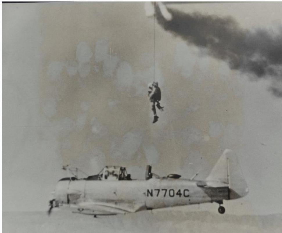
When the pilot activated the system by pulling a D-ring located between his thighs, the canopy was jettisoned and the rocket tilted upward and fired, extracting the pilot out of the cockpit as opposed to ejecting him.
