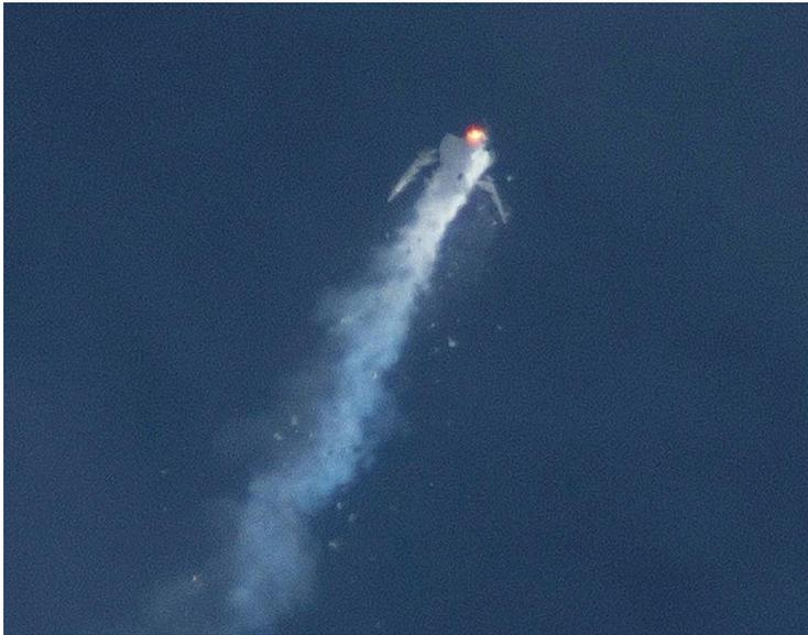
**Figure 2: SpaceShip Two Break up**
