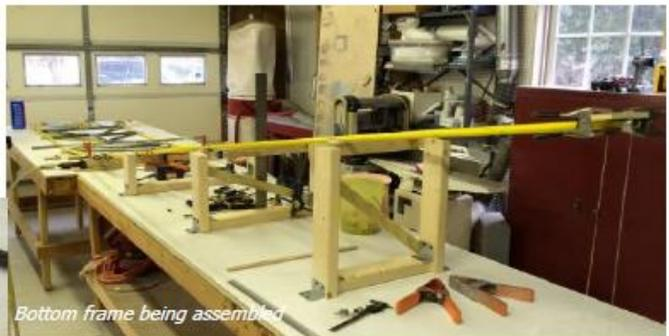
keep the bottom and top frames aligned to the long center line on the table. Once the basic placement was established I let the upright and diagonal tubes dictate the final assembly of the structure.
