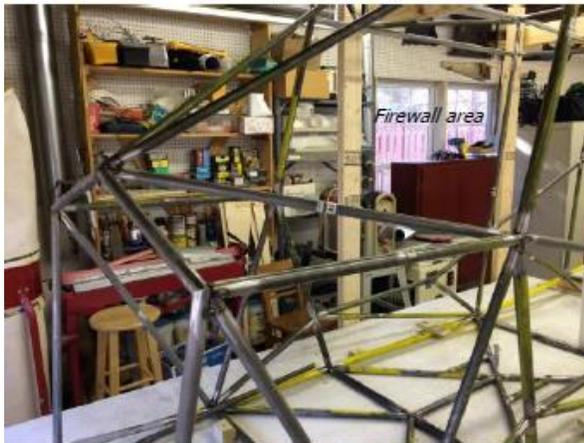
The forward fuselage and firewall area is definitely the most challenging, with more complex clusters. The 5 firewall tubes were numbered but were not found on the plan sheets. A little study and it became obvious which tubes were which. This is the only error or omission that I found in the drawings.
